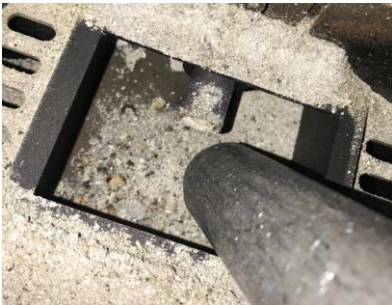
Example of a contaminated base
